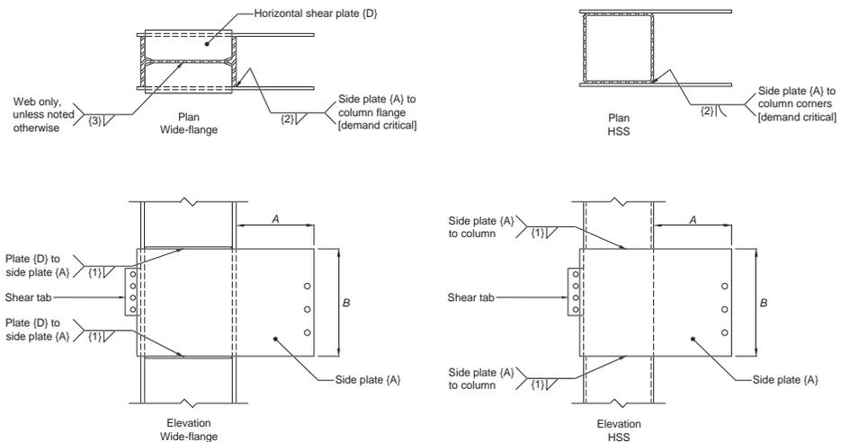
Fig. 11.11. One-sided SidePlate moment connection (A-type), column shop detail.
