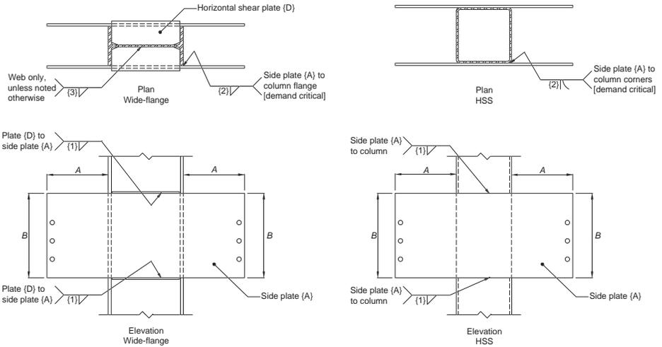
Fig. 11.12. Two-sided SidePlate moment connection (B-type), column shop detail.
