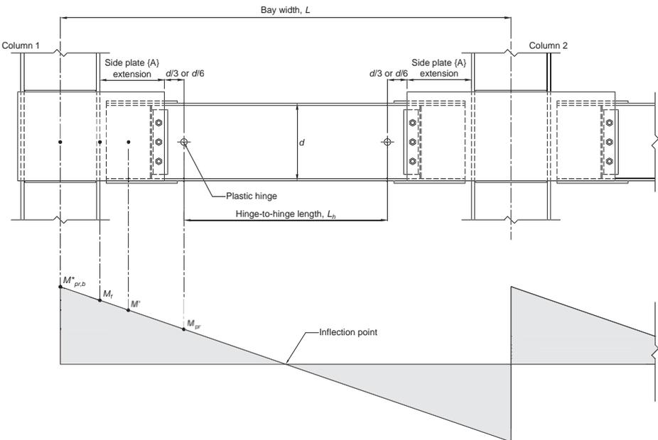
Fig. 11.6. Plastic hinge location and hinge-to-hinge length.
