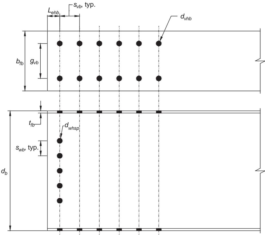
Fig. 13.4. Additional beam dimensions for double-tee connections.
