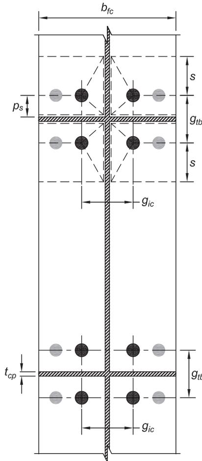
Fig. 13.8. Dimension for yield-line analysis of column flange.
