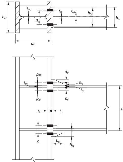
Fig. 6.3. Four-bolt stiffened extended end-plate (4ES) geometry.
