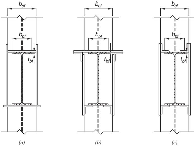
Fig. 11.9. Geometric compatibility (a) field-welded connection; (b) field-bolted standard connection (configuration A); and (c) field-bolted narrow connection (configuration B).
