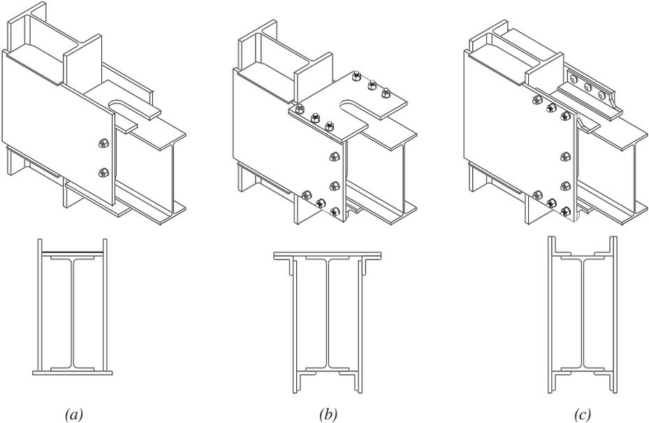
*Fig. 11.3. SidePlate field-welded and field-bolted connection comparison: (a) typical field-welded connection; (b) typical field-bolted standard connection (configuration A); and (c) typical field-bolted narrow connection (configuration B).*
