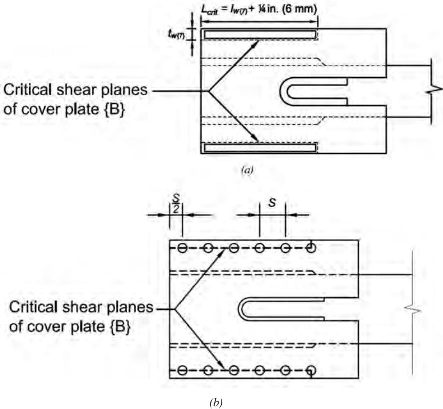
Fig. C-11.8. Critical shear plane of cover plate {B},
