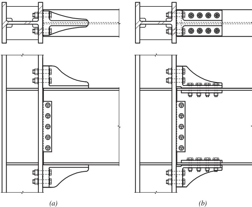
Fig. 9.1. Kaiser bolted bracket connection.
