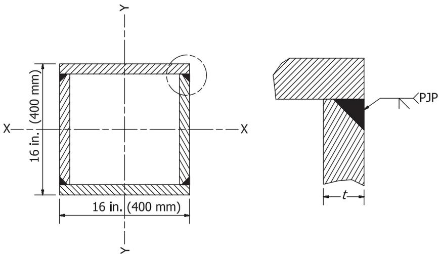
Fig. 10.5. Built-up box column flange-to-web connection detail.
