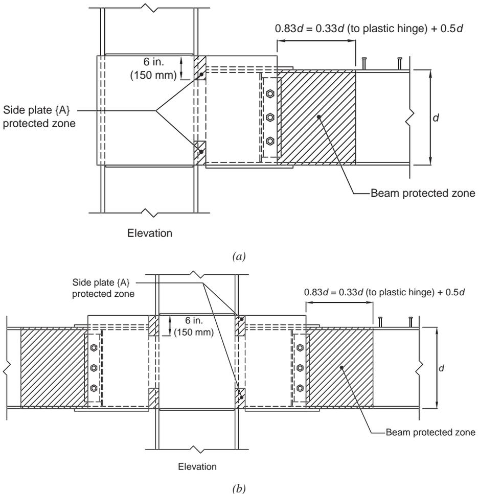
Fig. 11.7. Location of beam and side plate protected zones for the field-welded connection: (a) one-sided connection; (b) two-sided connection.
