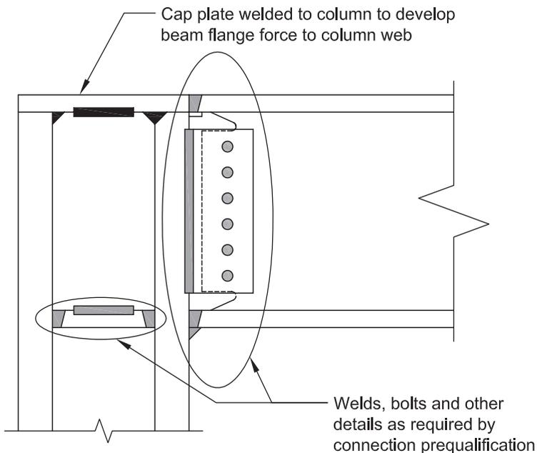
Fig. C-2.2. Example cap plate detail at column top for RBS connection.
