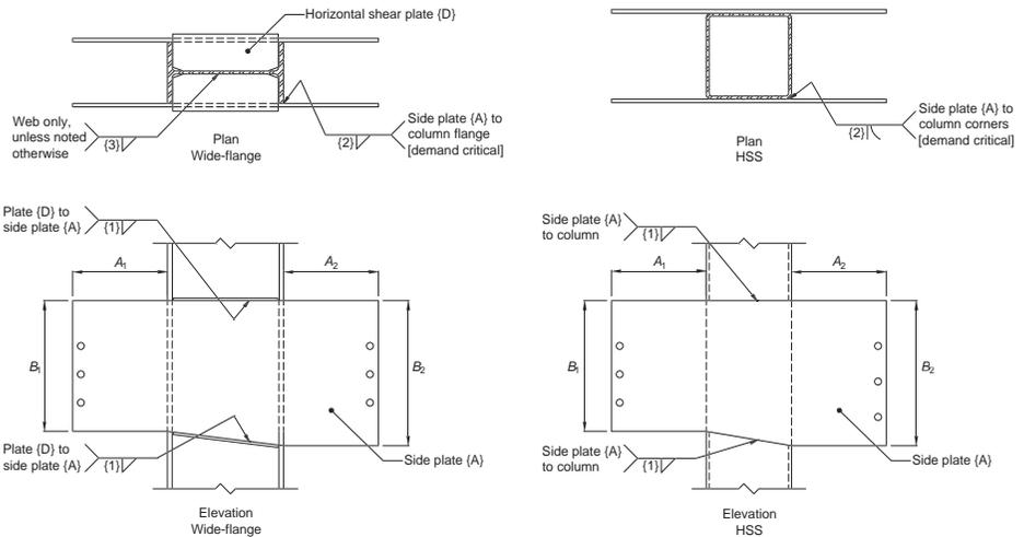
Fig. 11.13. Two-sided SidePlate moment connection (C-type), column shop detail.
