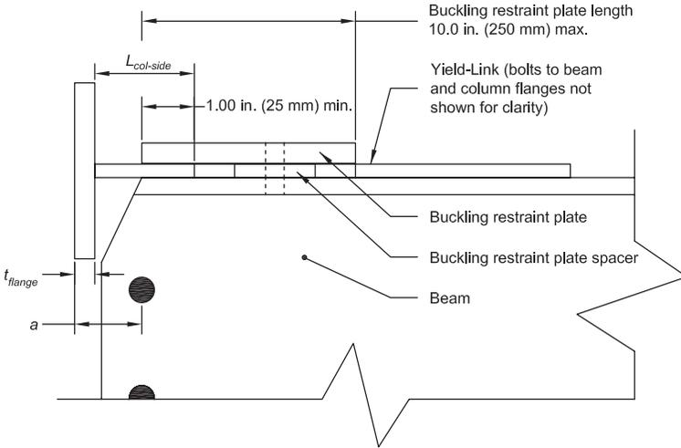
(c) Buckling restraint plate and Yield-Link  $L_{col-side}$  limitations
