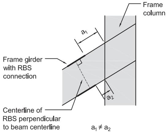
*Fig. C-5.2. Analytical studies (Kim et al., 2010) suggest that sloped frame beam with RBS centerline perpendicular to beam flanges perform better than if RBS centerline is parallel to column centerline.*
