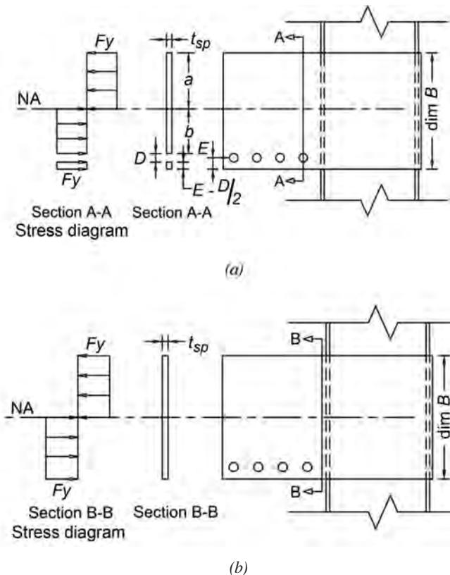
Fig. C-11.7. (a) Side plate {A} elevation view and stress diagram at the net section; (b) side plate {A} elevation view and stress diagram at the column face configuration A (standard).
