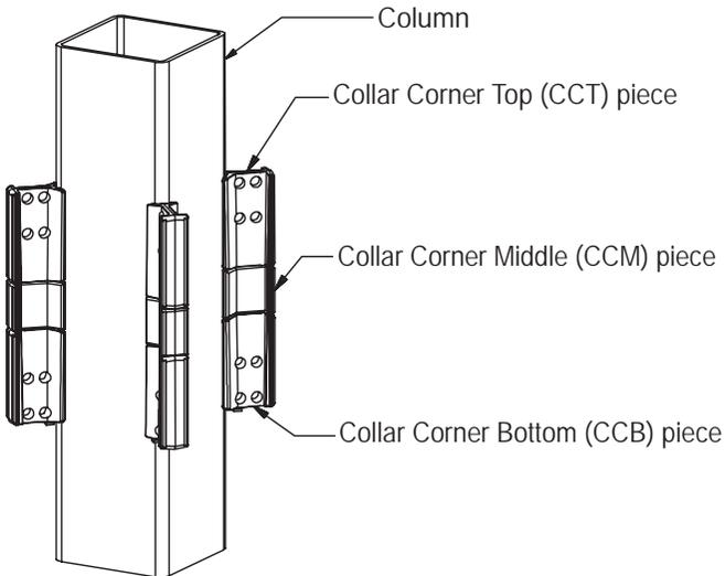
Fig. 10.2. Column with attached collar corner assemblies.
