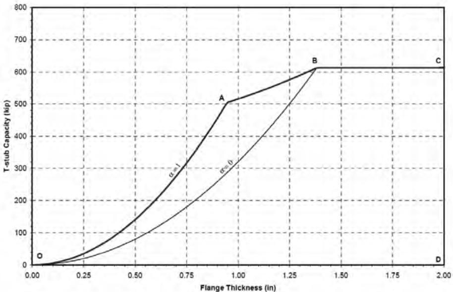
Fig. C-13.1. Relationship of T-stub capacity to flange thickness.
