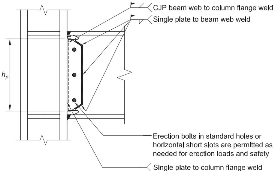
Fig. 8.2. General details of beam web-to-column flange connection.
