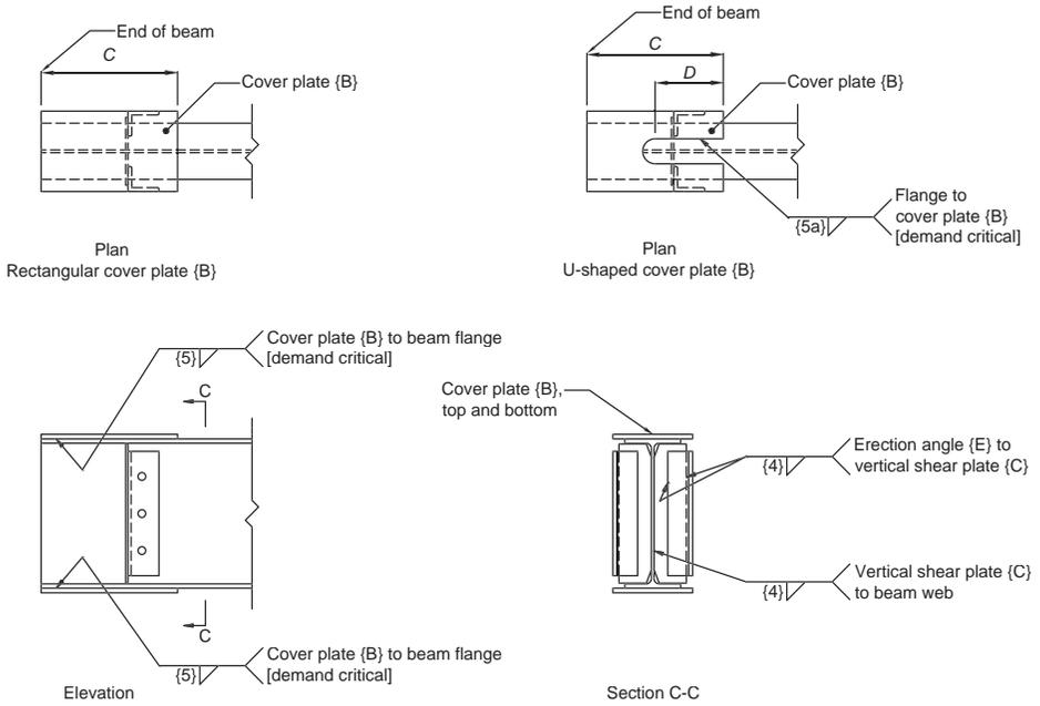
Fig. 11.14. Beam shop detail (field-welded).
