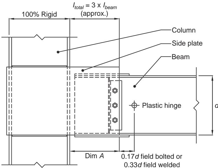
Fig. 11.17. Modeling of component stiffness for linear-elastic analysis.
