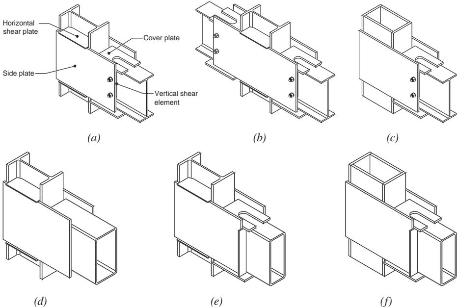
*Fig. 11.1. Assembled SidePlate uniaxial field-welded configurations: (a) one-sided wide-flange beam and column construction; (b) two-sided wide-flange beam and column construction; (c) wide-flange beam to either HSS or built-up box column; (d) HSS beam without cover plates to wide-flange column; (e) HSS beam with cover plates to wide-flange column; and (f) HSS beam with cover plates to either HSS or built-up box column.*
