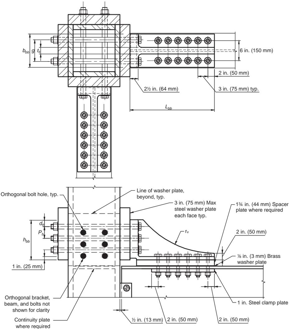
Fig. C-9.1. Box column connection detailing for KBB.
