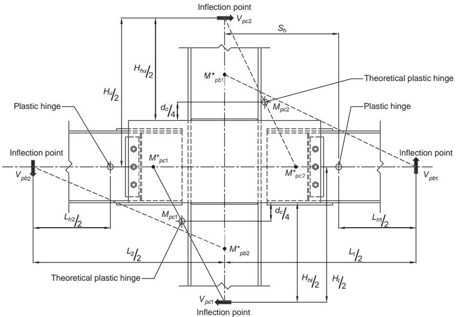
Fig. 11.10. Force and distance designations for computation of column-beam moment ratios.
