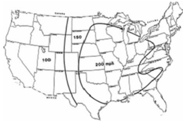
FIGURE C26.5-2 Tornadic Gust Wind Speed Corresponding to Annual Probability of 10^{-5} (Mean Recurrence Interval of 100,000 Years) (From ANSI/ANS 1983).
